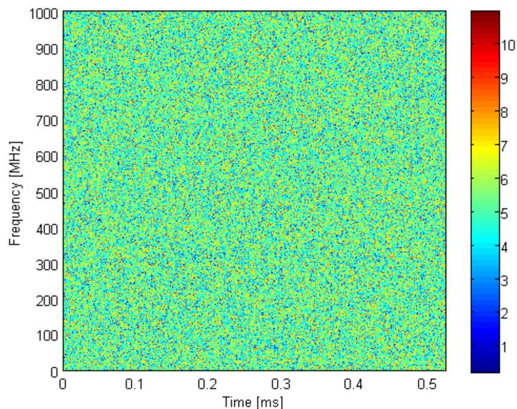
**Figure 3 Sonogram style frequency spectrum of a random noise signal**
