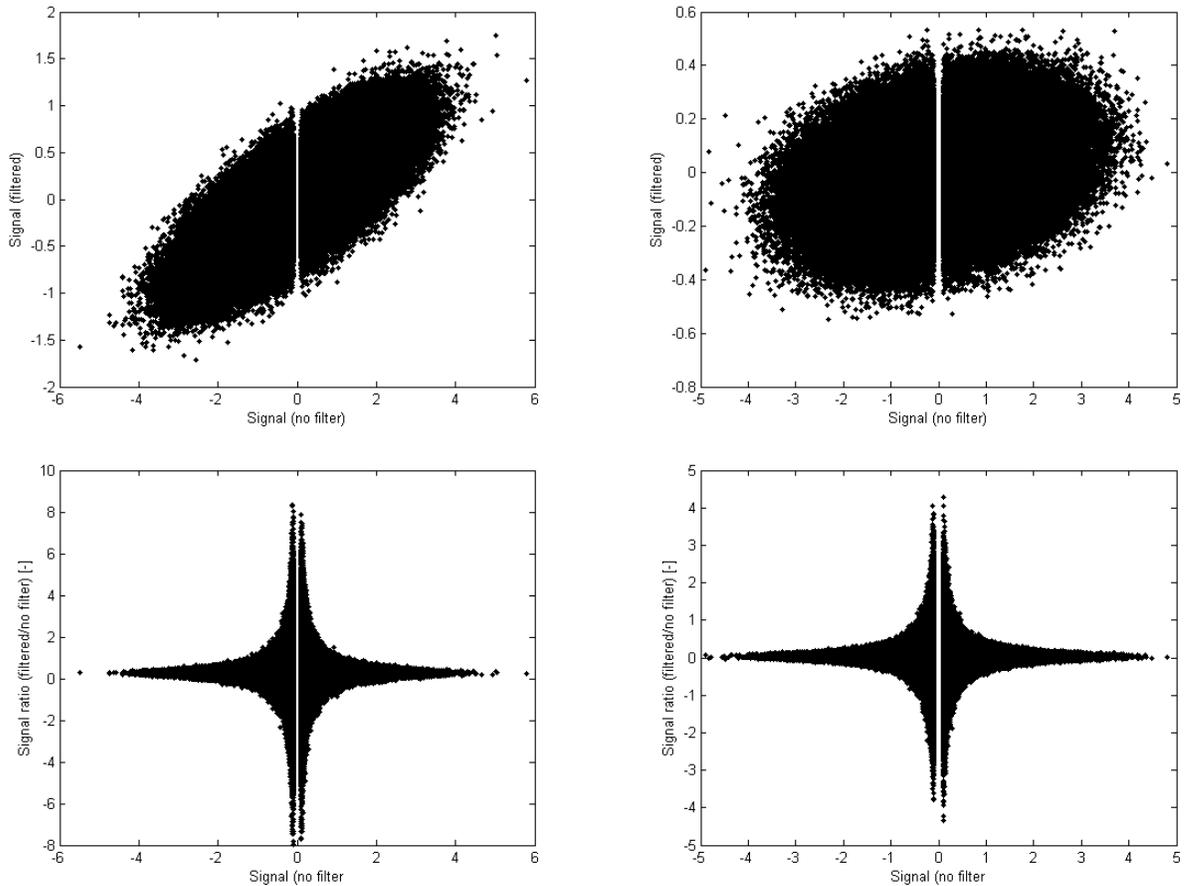
**Figure 6** Effect of low pass filtering on random data, using 3dB bandwidth of 900MHz (left) and 100MHz (right). Scatter plots of filtered vs. unfiltered data (top) and their ratio vs. unfiltered data (bottom).
