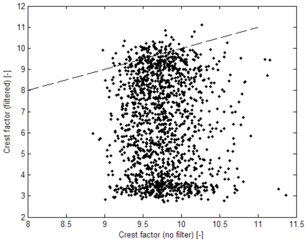
**Figure 9 Effect of low pass filtering on the crest factor of random data**
