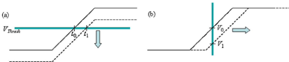
Figure 2: The effect of (a) amplitude noise on jitter and, (b), phase noise on voltage noise.
