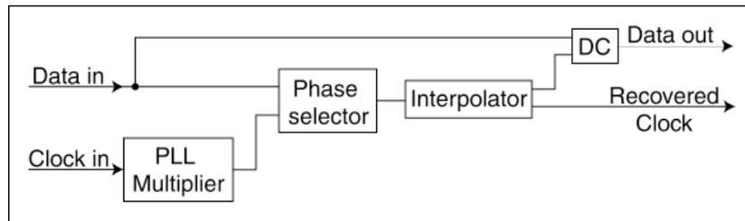
**Figure 7: Phase interpolator based receiver.**
