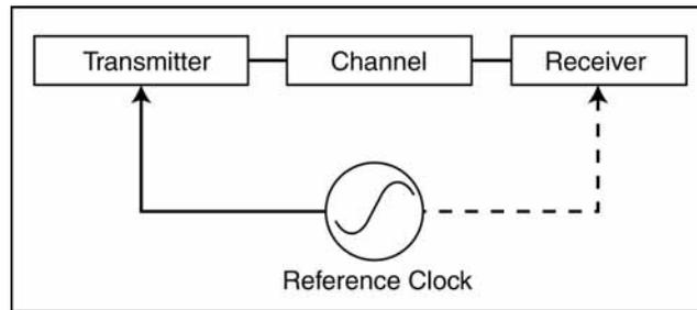
**Figure 1: Serial-data straw diagram emphasizing the role of the reference clock.**
