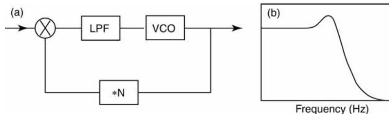
**Figure 6: PLL Multiplier (a) block diagram, (b) frequency response.**
