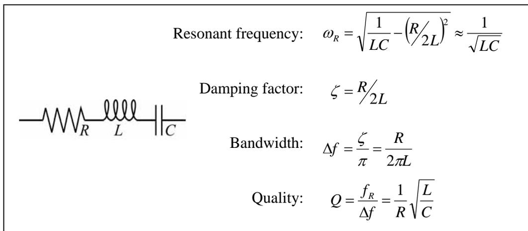
**Figure 2: A simple oscillator and typical parameters.**
