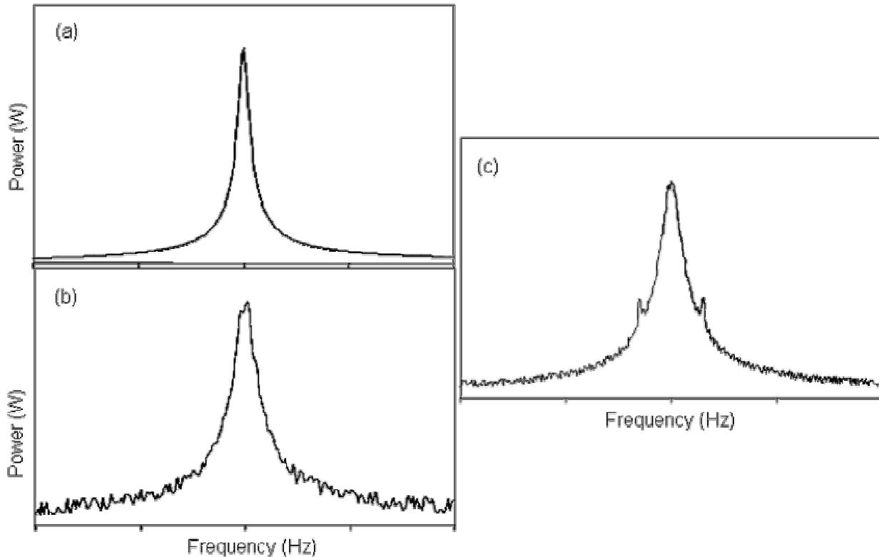
**Figure 5: Oscillator or clock signal in the frequency domain, (a) an ideal Lorentzian resonance, (b) with white noise, (c) with spurs from crystal vibrations.**
