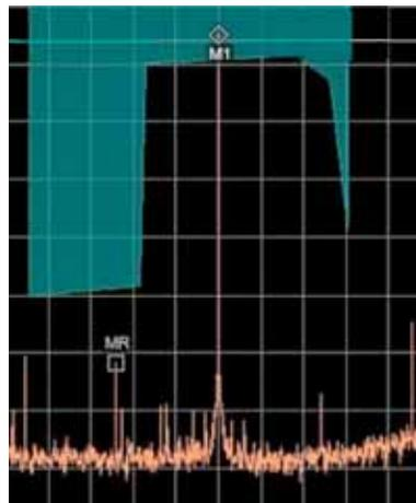
**Figure 4: Spectrum of an oscillator as it settles.**
