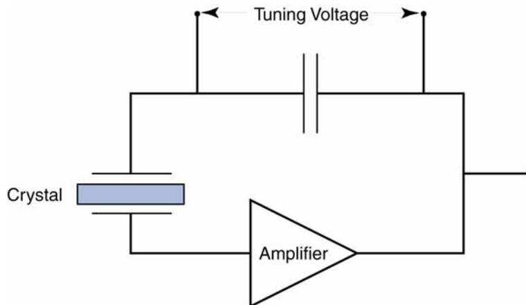
**Figure 3: Crystal oscillator [circuit diagram]**
